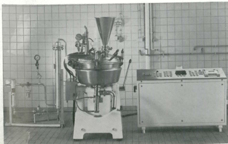
Console mounted control panel with operating push buttons and programme card feeder, water dosing and temperature indicator
